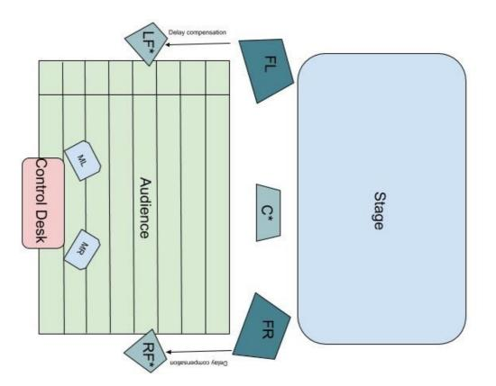
FL - Front Left Speaker FR - Front Right Speaker C\* - Center LF\* - Left Fill RF\* - Right Fill RF\* - Right Fill ML/MR\*\* - Control Monitors
